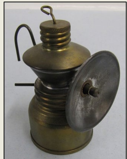
Example of a miners' carbide lamp showing the reflector plate (similar to The Mystery Artifact) attached to two chambers: the upper chamber that held water and a lower chamber that held the calcium carbide.
