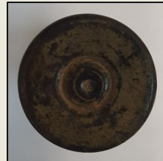
Externally primed .45-70 Govt. cartridge with no headstamp.
