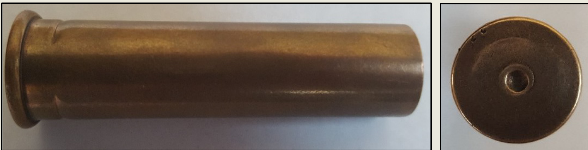
Unmarked internally primed .45-70 Govt. cartridge with a wide space between crimps on the lower case.
