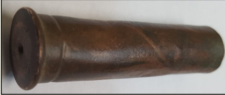
Internally primed .45-70 Govt. cartridge with faint F/C/9/78 headstamp with a narrow space between crimps on the lower case.
