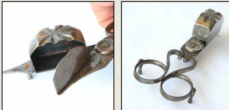
Figure 3. Left: View showing how the handles open the box to put over the candle wick and flame. Right: View showing two of the three metal feet and the scissor handle mechanism.
